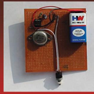
The final circuit with a battery to power the circuit. The positive terminal of the lead acid battery is connected to the tab of the transistor and the negative terminal to pin 2 of the transistor. Copper wires are used to connect the lead acid battery to the transistor with a nichrome loop in series to act as the heating element
