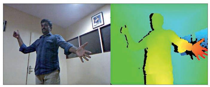
Here we see two different images of the same scene to give you an idea of how the Kinect perceives the world in front of it. On the left is the output from its VGA camera, which is close to how we see things in our surrounding. However, the image on the right shows the depth map of the same scene.
