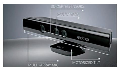
Here's a pic that highlights the main aspects of Kinect. It has a 3D depth sensor, RGB camera, motorized tilt and a multi-array mic.
